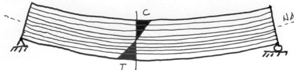
In the initial unloaded state, all transverse sections are parallel.
