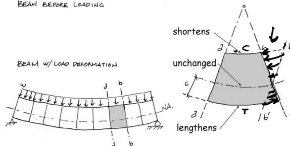
Notice that by the geometry of the curved member the top edge is shortened and the bottom edge is lengthened. Only the neutral axis remains its original length.
