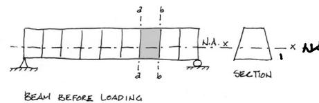
The application of load causes the member to bend in a curve. This means the initial parallel plane sections, while remaining plane, now follow the radii of the curves.
